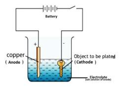
Electroplating is the process of plating one metal onto another using electrolysis. Here is how it works (example of coating brass with copper):
